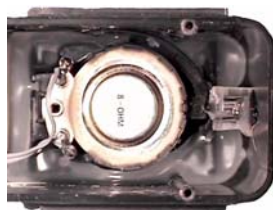
Mounting speaker in hood of engine using a metal grill for the exhaust.
