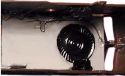
Sometimes it is necessary to make a small baffle inside an open shell. Again, make sure all areas that encase the backside of the speaker are closed.
