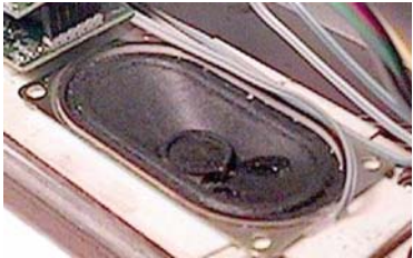
Using the fuel tank as a speaker baffle is quite easy. In this case the speaker emanates sound into the body.
